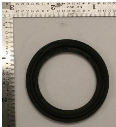
Figure 1: The diameter before and after soaking in methanol was measured using a high-resolution image taken with a DSLR camera.
